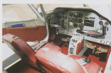
Left: ... as does a modern panel, but, rudder straps, odd yokes, mag switches and other details give the game away—it's still a Yak.
