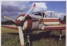
Below: westernised paint scheme and interior, plus 400 hp and 3-blade prop, and Yak-18T has forties opulence.
