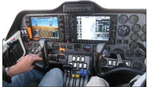
**We flew the developmental aircraft that had both a G950 (essentially a G1000 system without an integrated autopilot) and full analog gauges. This led to a cluttered panel. Production models will have either analog or G950 with some analog backups. The yellow knobs on the power quadrant are carb heat, as Rotax engines adjust mixture automatically.**
