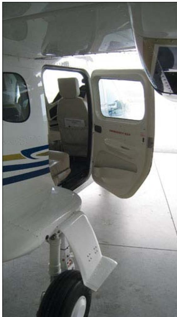
**Using the rear door requires a somewhat awkward maneuver under the wing and around the gear door and housing. Once inside, the rear seating and baggage area feels bigger than any comparable aircraft.**
