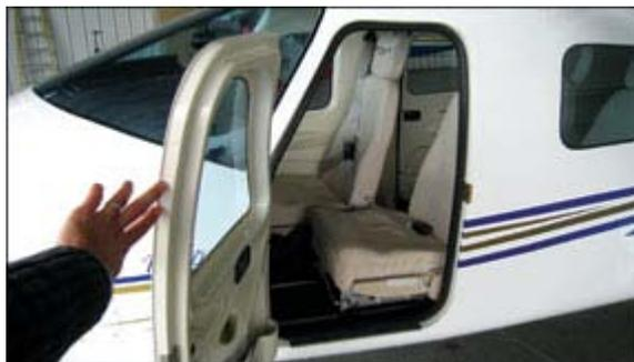
**Getting in and out of the front seats is a breeze, even with a front door on only one side. All four seats adjust up and down, as well as fore and aft. Structurally, the P2006T is surprisingly beefy, but interior finish and parts are quite lightly made. The conventional aluminum construction should make for simple repairs.**
