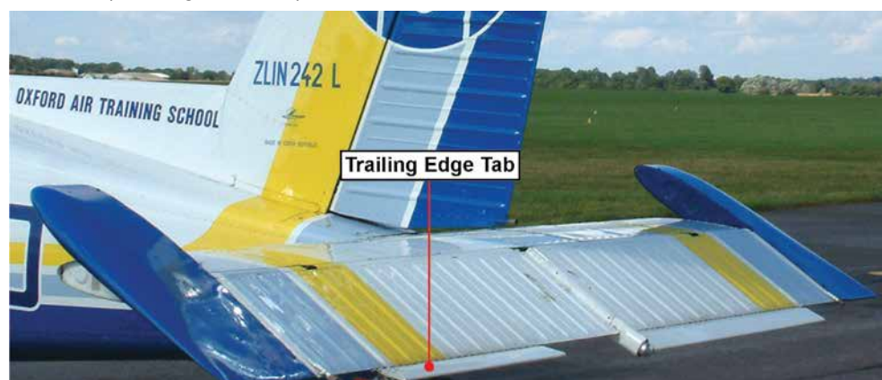
Figure 12.27 Trailing edge tabs, in this case a balance tab. The other tab is the elevator trim tab.
