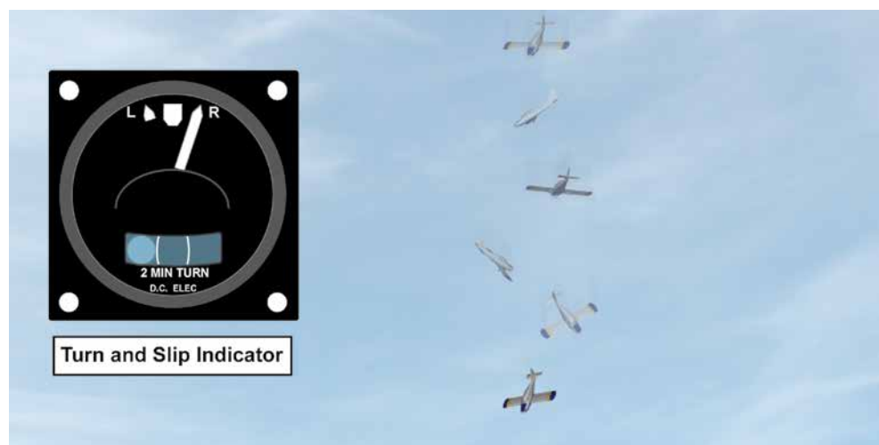
Figure 13.30 The turn needle will always indicate the direction of spin.
