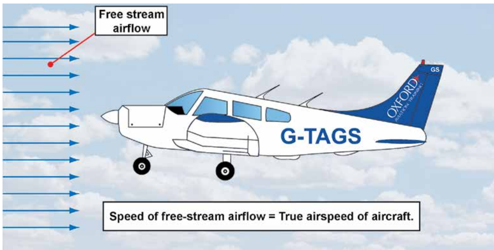
Figure 4.13 The speed of the free-stream airflow is the same as the aircraft's true airspeed.
