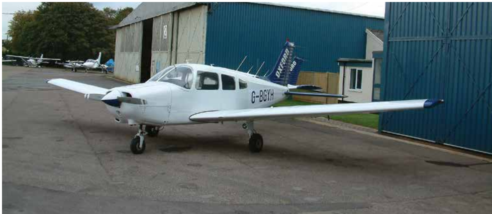
Figure 11.22 Positive dihedral on the Piper PA28 Warrior.
