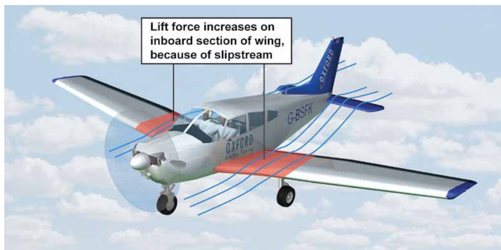
Figure 11.29 High power settings at low forward speed reduce lateral stability.
