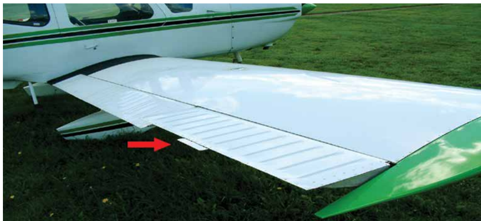
Figure 12.35 A fixed trim tab on a aileron.
