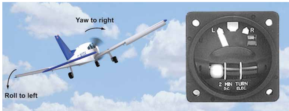
Figure 12.10 Adverse yaw. Here the aircraft is rolling to the left and yawing to the right. Notice the position of the ball showing that the aircraft is out of balance.
