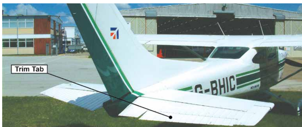
Figure 12.36 An adjustable trim tab fitted to the elevator of a Cessna.
