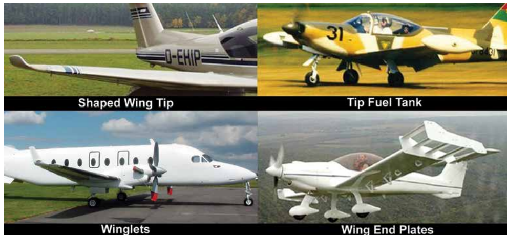
Figure 5.25 Wingtip shapes designed to reduce wingtip vortex strength.
