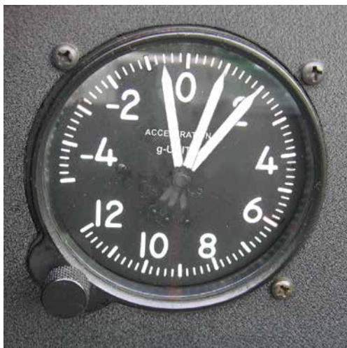
Figure 14.8 An accelerometer, or g-meter, which records load factor.
