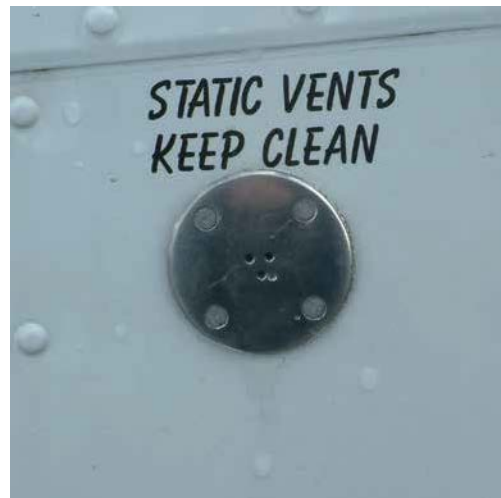
Figure 4.16 A Static Vent.
