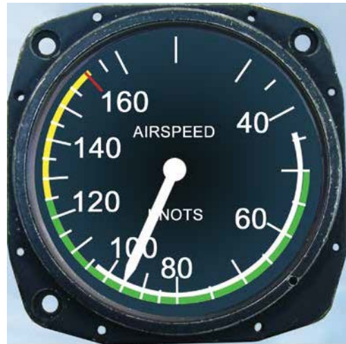
Figure 4.15 An Airspeed Indicator (ASI) indicating 95 knots.
