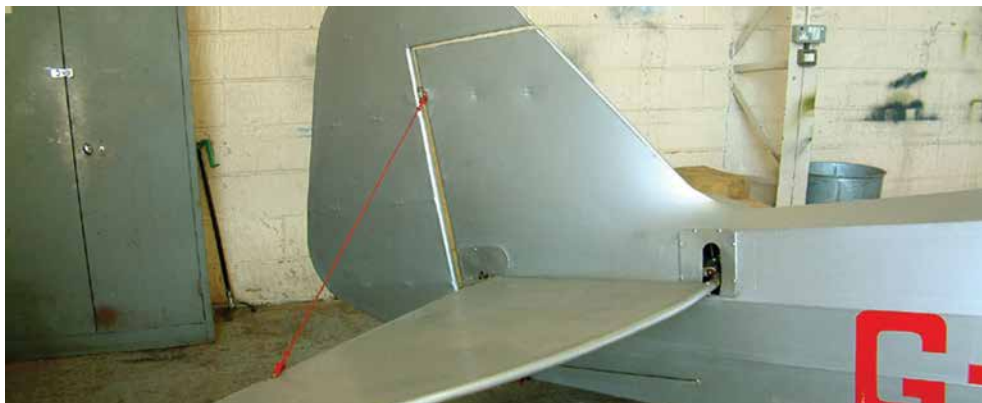
Figure 12.41 A variable incidence tailplane.
