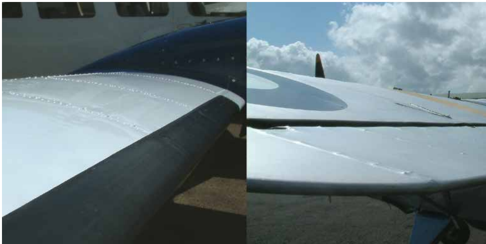
Figure 5.3 The surface area and the surface finish affect skin friction drag.
