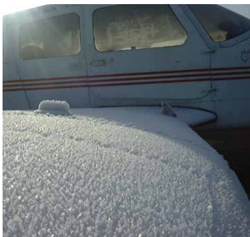
Figure 13.18 Frost, snow and ice on the wings increase stall speed.
