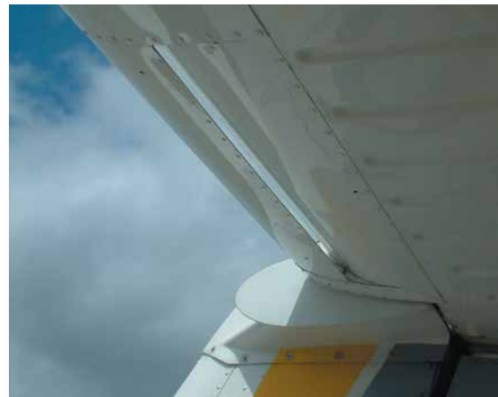
Figure 10.26 The tailplane is an aerofoil and may be fitted with slots.
