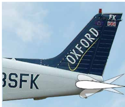
Figure 12.3 A stabilator or all-moving (flying) tailplane.
