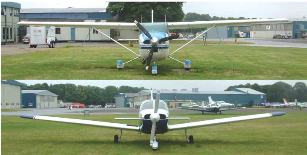
Figure 11.23 The difference in dihedral between low and high wing aircraft.
