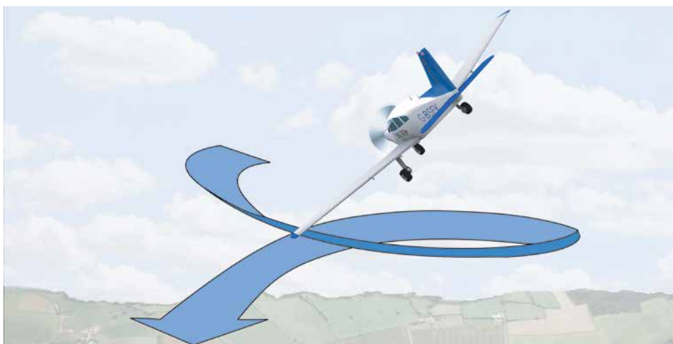
Figure 12.9 The secondary effects of both rudder and ailerons induce rolling and yawing actions, in the same direction, which mutually reinforce each other and lead to a spiral dive.
