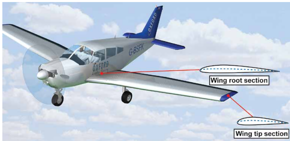
Figure 13.12 Variation in aerofoil section along the wing.
