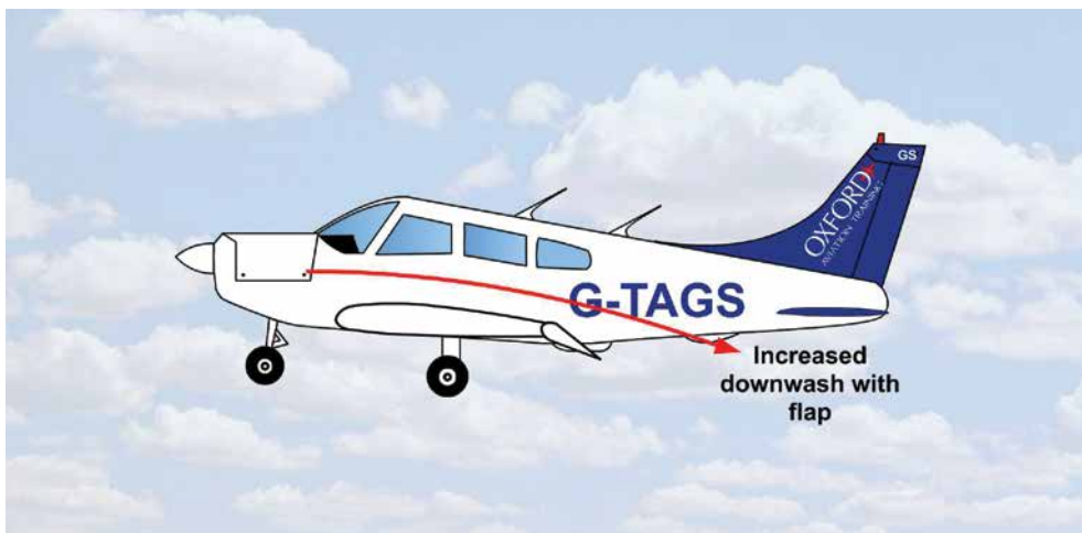
Figure 10.17 Lowering flap will modify downwash and influence an aircraft's trim in the pitching plane.
