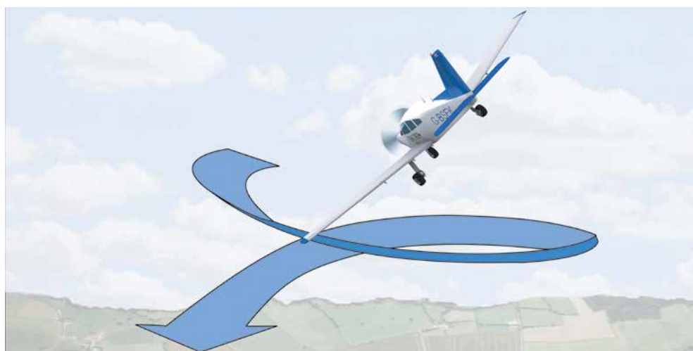
Figure 11.35 Rolling and yawing actions mutually reinforce themselves in the same direction and lead to a spiral dive.
