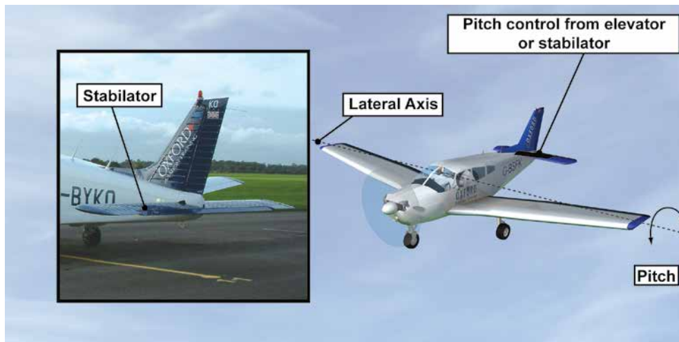
Figure 12.7 The elevator controls the aircraft in pitch.
