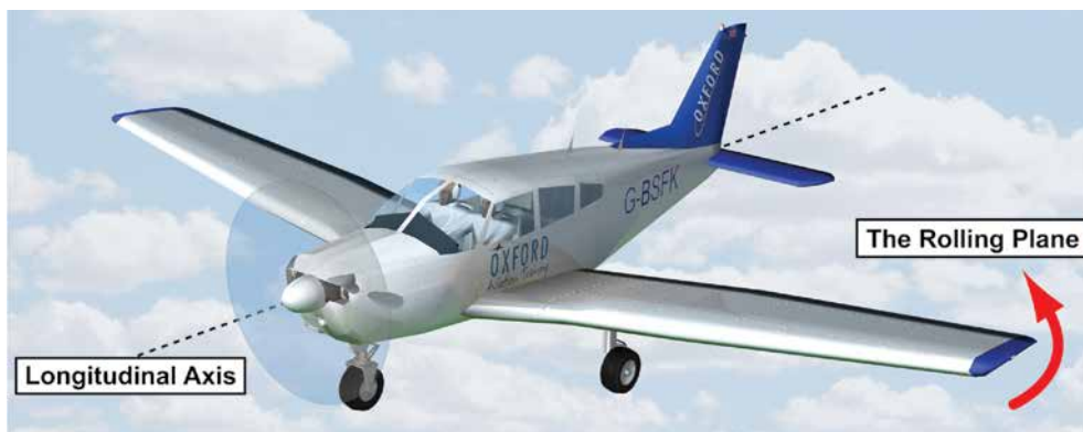
Figure 11.15 Lateral Stability is stability in roll about the longitudinal axis.
