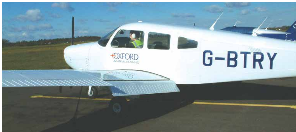
Figure 14.13 The flaps and their operating mechanism are not designed to withstand the aerodynamic loads which occur at high cruising speed.
