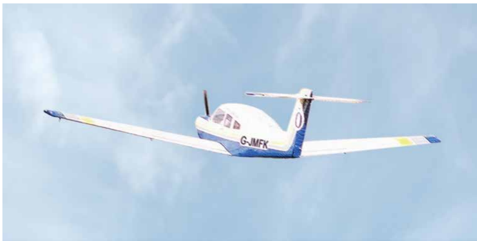
Figure 14.15 Gear is retracted when safely airborne.
