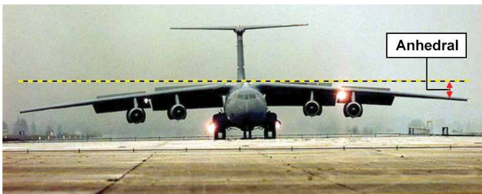
Figure 11.27 Anhedral reduces lateral stability.
