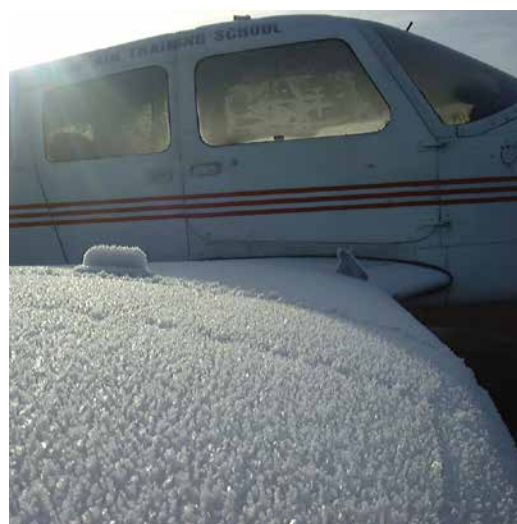
Figure 2.17 Wing contamination will degrade an aerofoil's lift-generating properties and increase Take-Off Distance Required. Ice and snow will also significantly increase weight.
