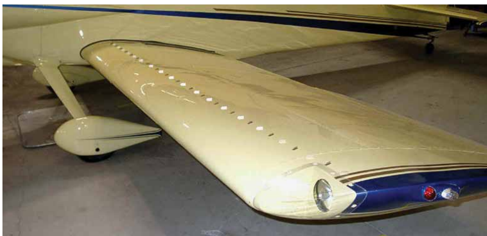
Figure 13.14 Vortex generators delay separation of the boundary layer.
