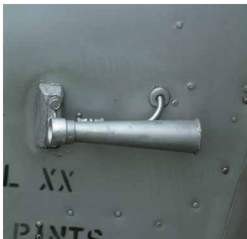
Figure 4.12 Venturi Tube fitted to Auster J6.
