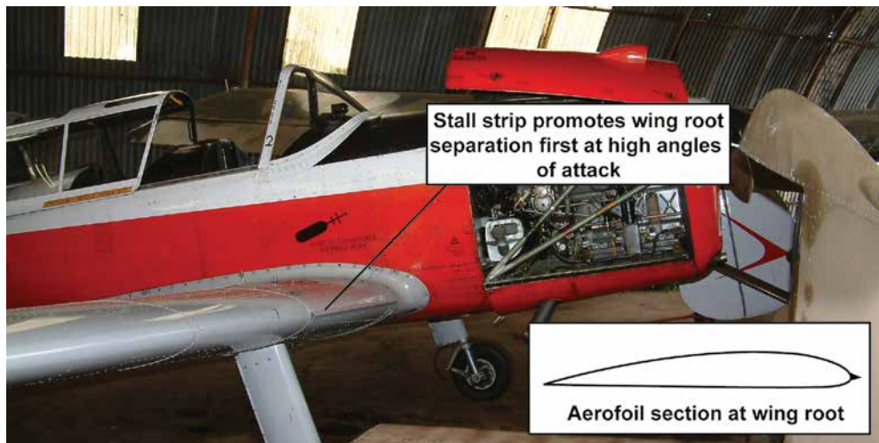
Figure 13.13 Stall strips help to ensure that the wing root stalls first.
