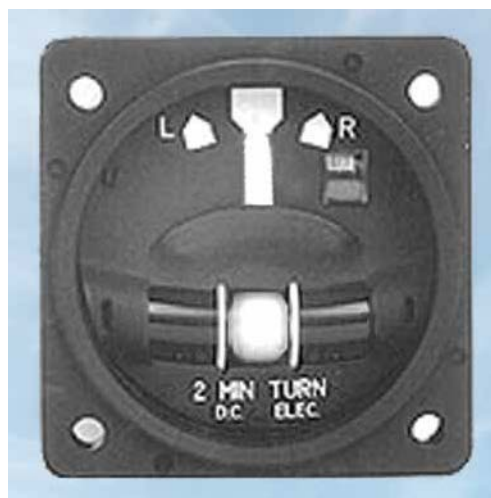
Figure 12.6 The rudder is primarily used to keep the aircraft in balanced flight with the ball "in the middle".
