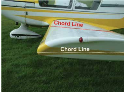
Figure 5.24 Washout refers to the reducing angle of incidence from root to tip. Washout also helps to reduce induced drag.
