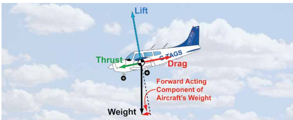
Figure 4.10 A constant-speed descent, with all principal flight forces in equilibrium.
