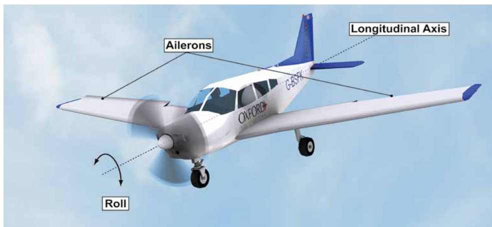
Figure 12.8 Control in roll is achieved with the ailerons.
