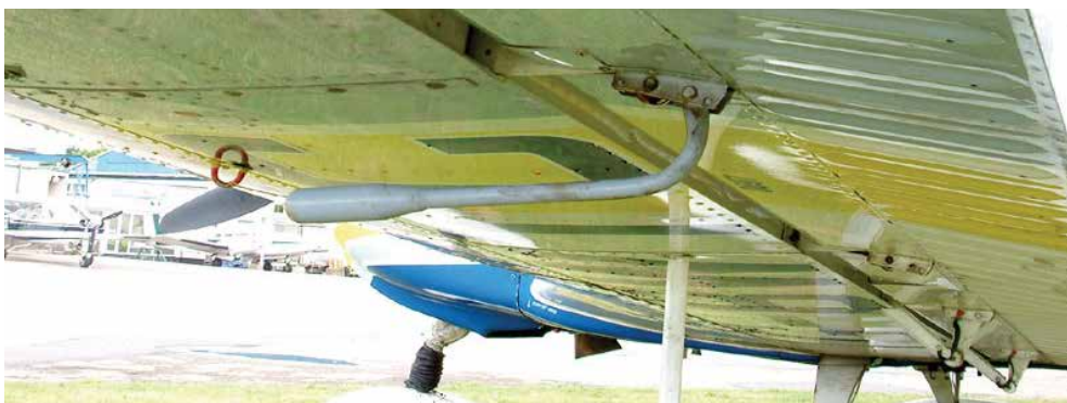
Figure 12.34 The mass balance fitted to the ailerons of a Zlin 242L.
