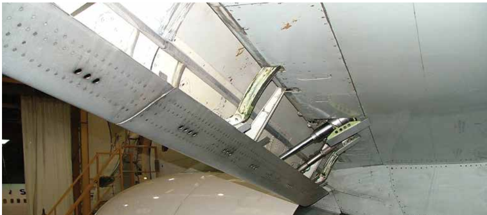
Figure 10.23 A typical leading edge flap on a jet transport aircraft.
