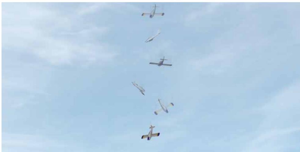
Figure 13.27 The spin is a state of stalled flight with the aircraft in a steep descent, yawing, rolling and pitching at the same time.
