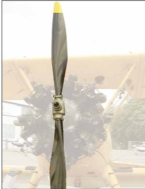
Figure 8.15 A propeller blade is twisted along its length with the blade angle decreasing from hub to tip.
