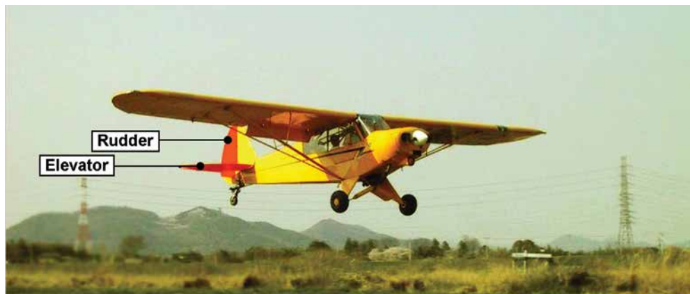
Figure 12.19 Only the rudder and elevator benefit from the propeller slipstream effect.
