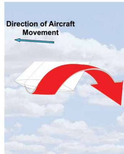
Figure 5.17 The wingtip vortex is particularly large and strong.
