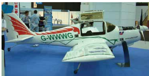
Figure 5.4 Composites materials produce continuous smooth structures which have low skin-friction drag.
