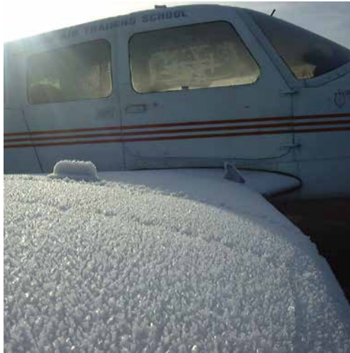
Figure 5.5 The surface area and the surface finish affect skin friction drag.
