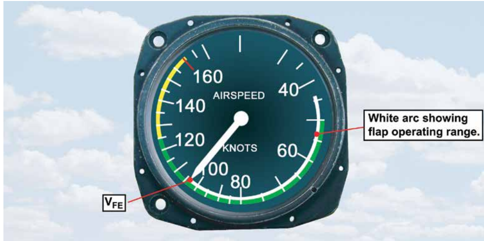
Figure 10.21 The flaps can safely be operated if the aircraft's speed is within the white arc.
