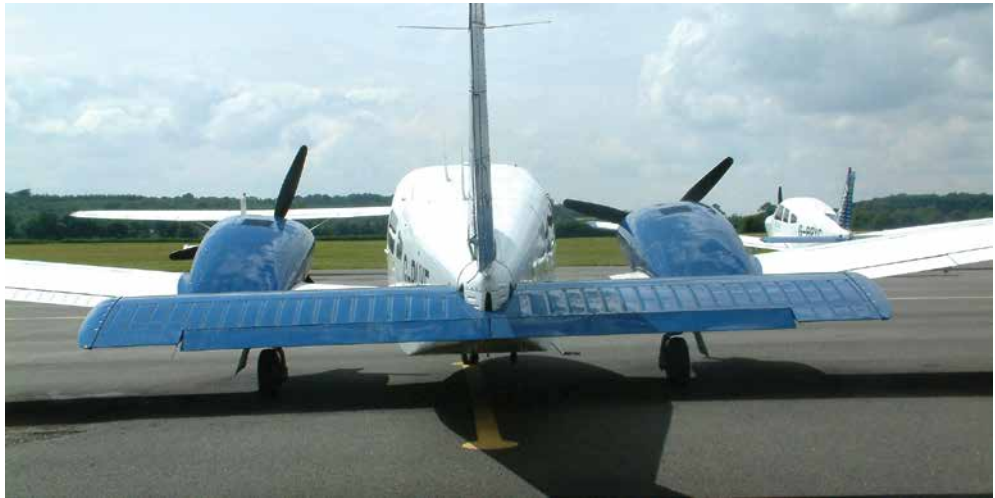
Figure 12.30 Anti-balance tabs are most commonly found on aircraft with all-flying tailplanes or stabilators.
