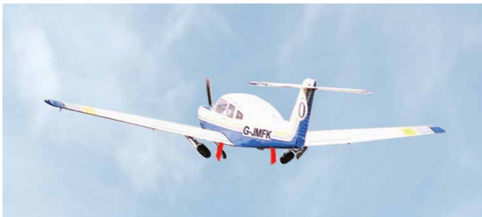
Figure 14.16 Gear doors are not able to withstand large aerodynamic loads.
