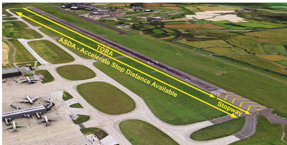
Figure 2.4 ASDA (Acceleration Stop Distance Available) = TORA + Stopway
