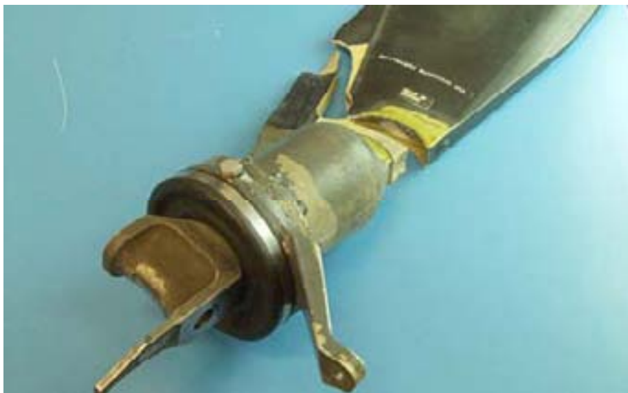
Figure 2: The fractured main rotor blade, VH-OHA
