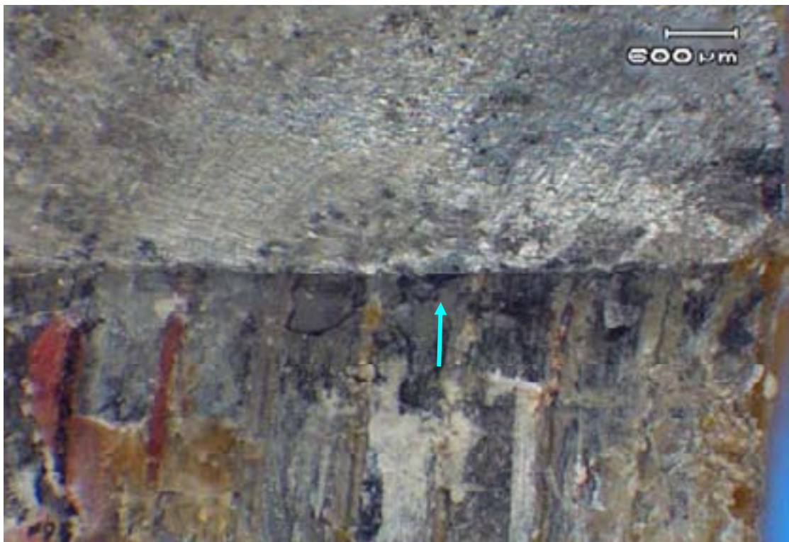
Figure 9: Extended focus light microscope image of the first initiation site
