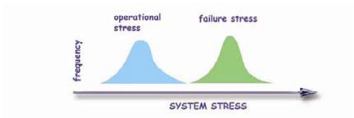
Figure 18: Schematic illustration of the probability of failure under conditions of variable operational stress and failure stress – no failure condition
