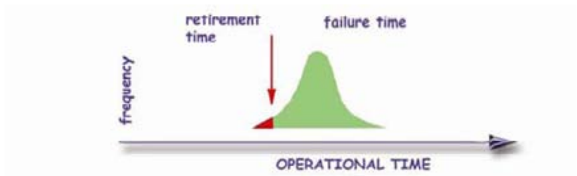
Figure 17: The relationship between retirement time and failure time that results in the failure of a number of components of a particular configuration
