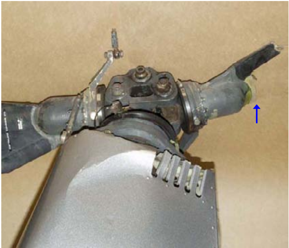
Figure 1: The recovered main rotor head assembly, VH-OHA
