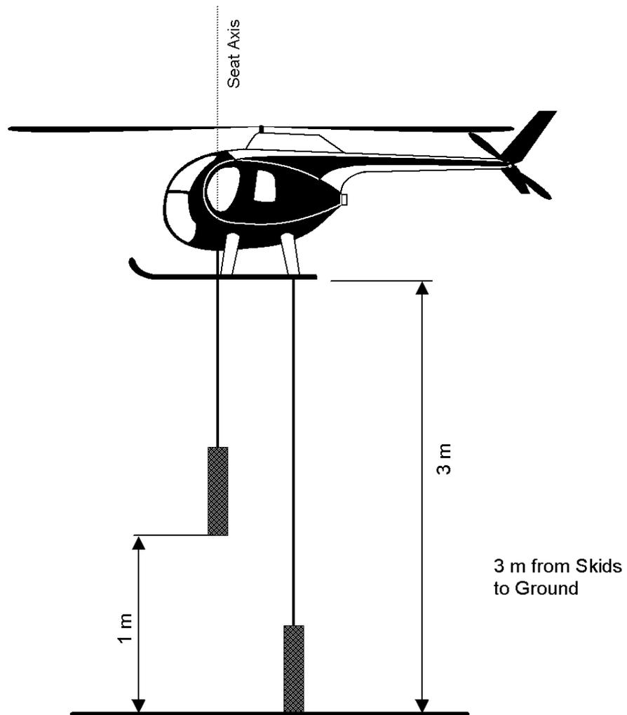
It is essential to understand that from one helicopter to another, the short rope will differ in size. The objective is to have 1 metre difference between the bottom of the two weights.
