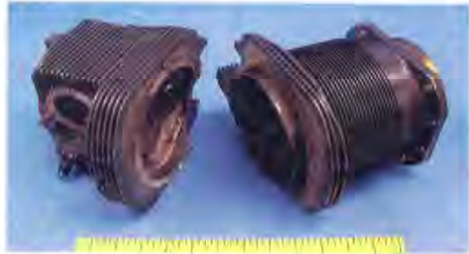
Figure 2—Head-to-barrel separations are not limited to Continental engines. Here's a Lycoming cylinder that lost its head. (NTSB photo.)
