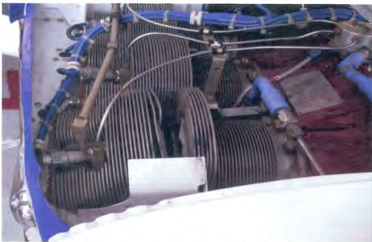
Figure 3— Head-to-barrel separation of #5 cylinder on a Continental TS10-520 engine.
