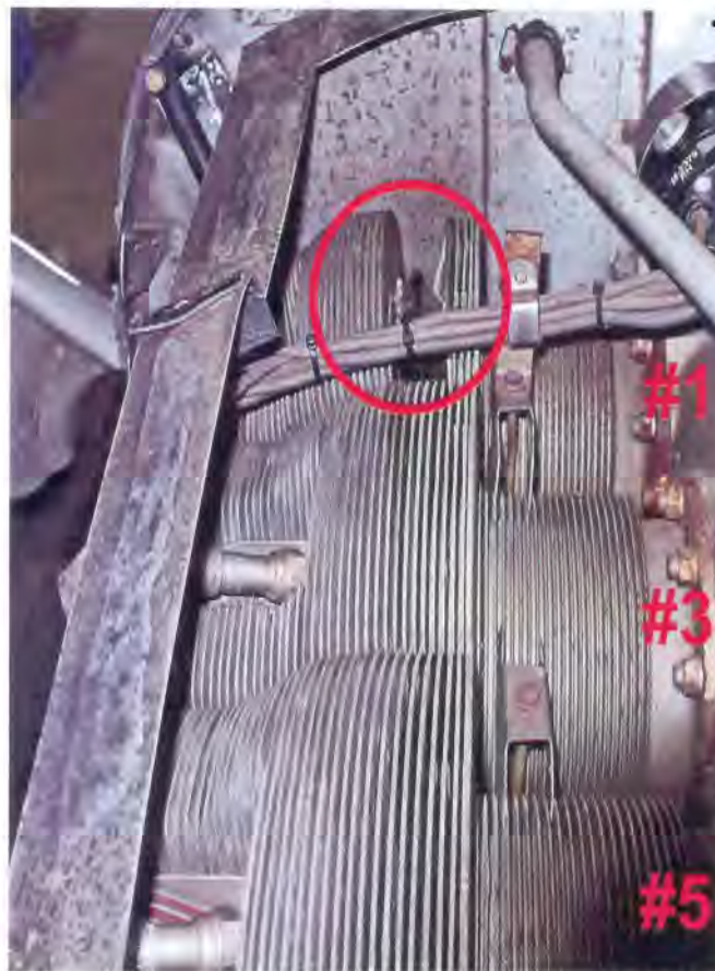
Figure 1— The #1 cylinder head on this TCM O-470-U engine suffered a catastrophic fatigue failure in flight. The #3 cylinder suffered a similar failure about an hour later!
