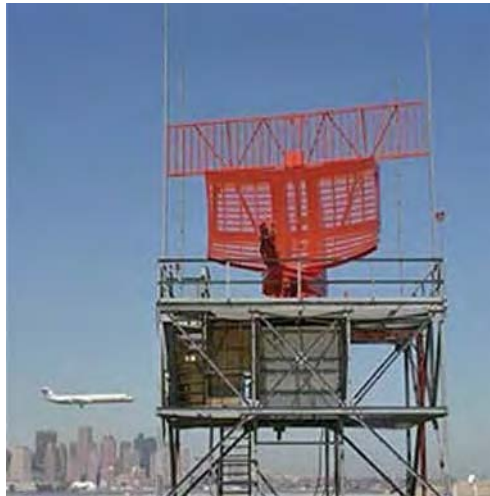
Figure 19.1 A terminal area surveillance radar at an airport. The radar head makes approximately 10 rotations per minute.
