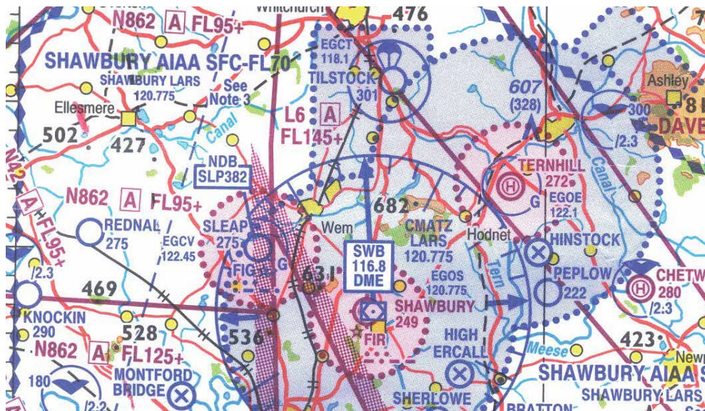
Figure 14.6 Shawbury is equipped with VOR/DME on 116.8 MHz (2010).
