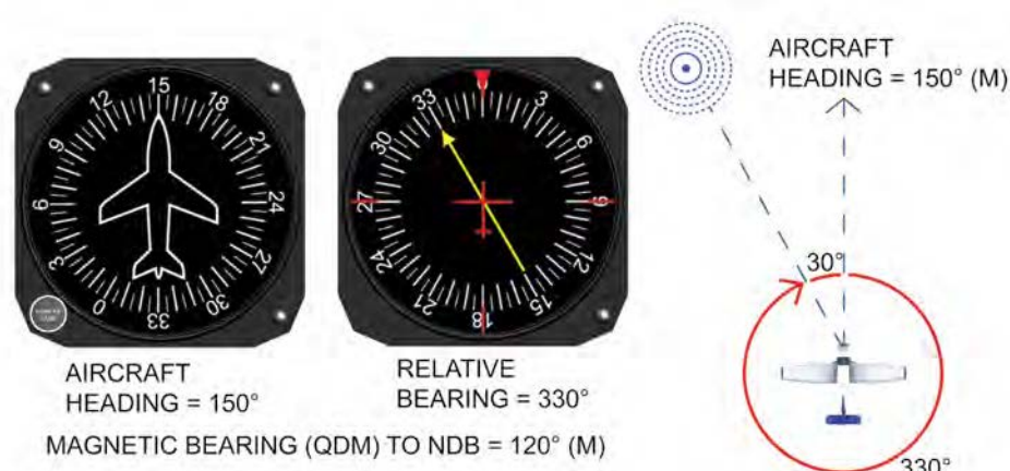
Figure 16.8 A DI used in conjunction with an RBI to determine the QDM to the NDB.
