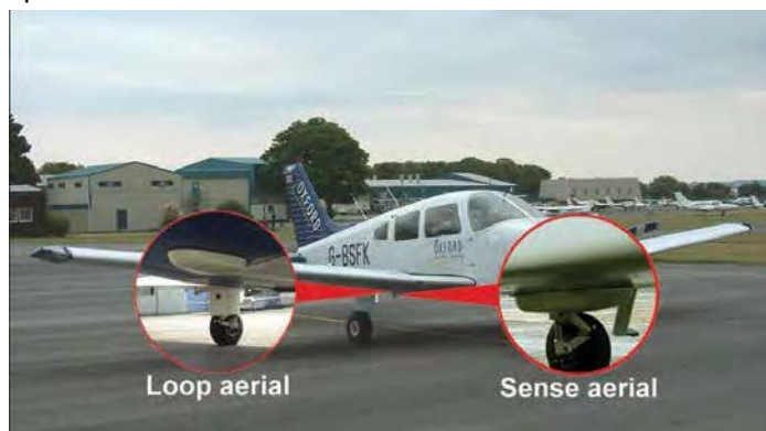
Figure 16.5 An ADF Loop and Sense Aerial.
