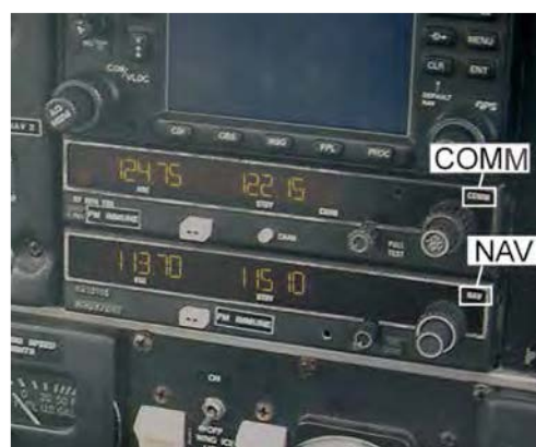
Figure 17.6 The VOR receiver (NAV) alongside the VHF voice communication receiver (COMM).
