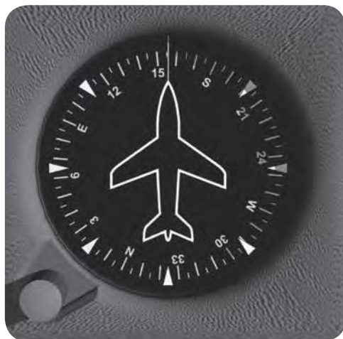
Figure 3.19 A Direction Indicator.
