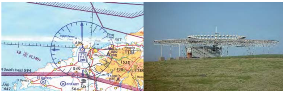
Figure 17.4 The Strumble VOR/DME, near Fishguard (Photo by courtesy of Mr Trevor Diamond.)
