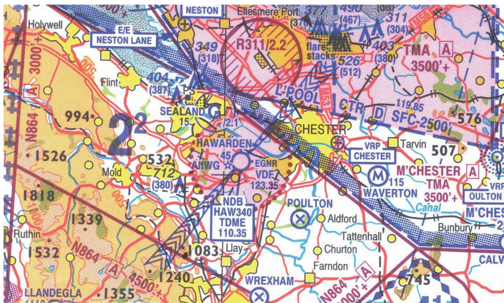
Figure 14.5 Hawarden is equipped with an NDB and a DME beacon.
