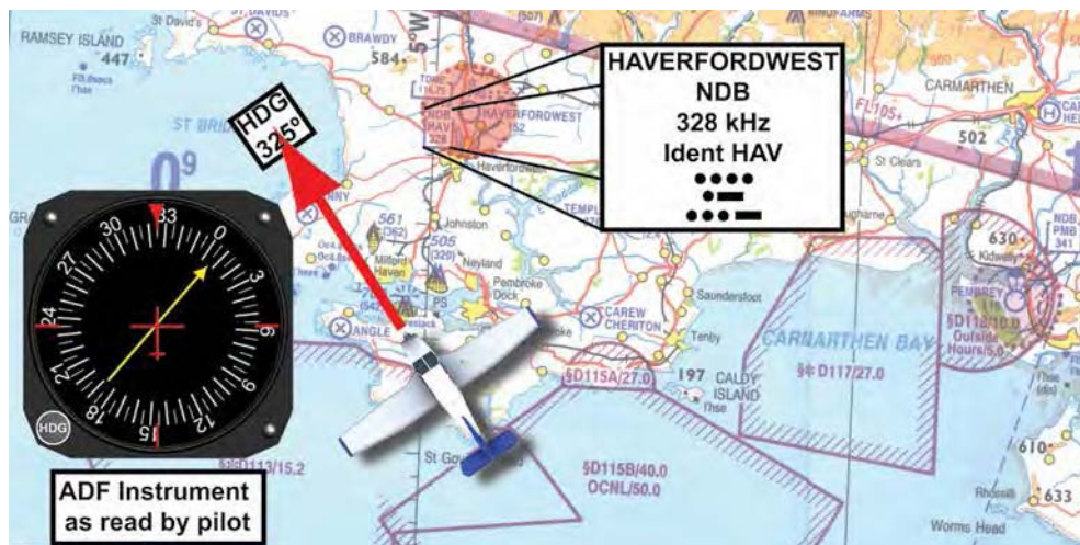
Figure 16.10 An aircraft on heading 325°, with the ADF display showing a TQ bearing of 008°, and a FROM bearing (radial) of 188°. The RBS of the ADF display is aligned with the DI and therefore reads the QDM directly.
