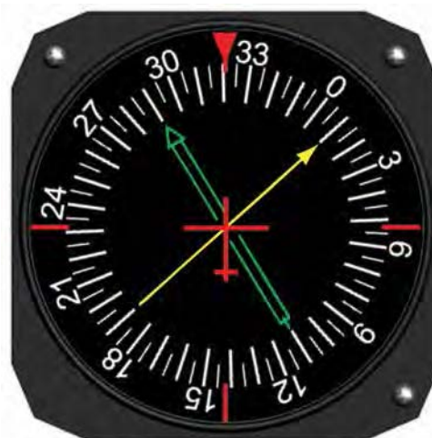
Figure 16.12 A twin - needle RMI with ADF and VOR indicators.
