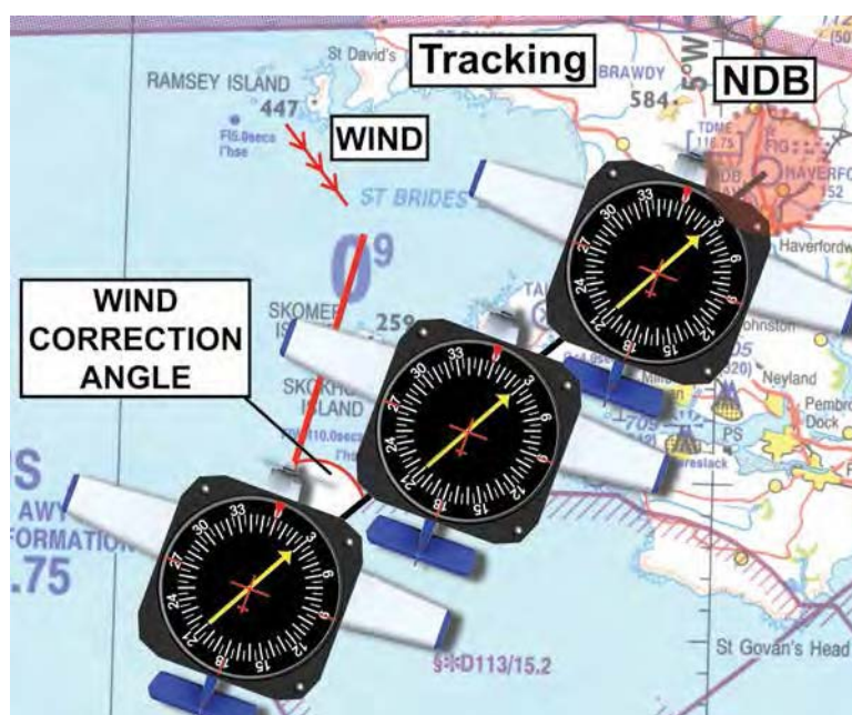
Figure 16.14 Tracking directly towards an NDB, compensating correctly for drift, and maintaining a constant QDM, with a relative bearing of 030° on the RBI.
