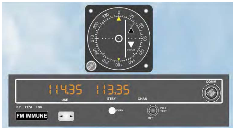
Figure 17.1 VOR Receiver and Display.
