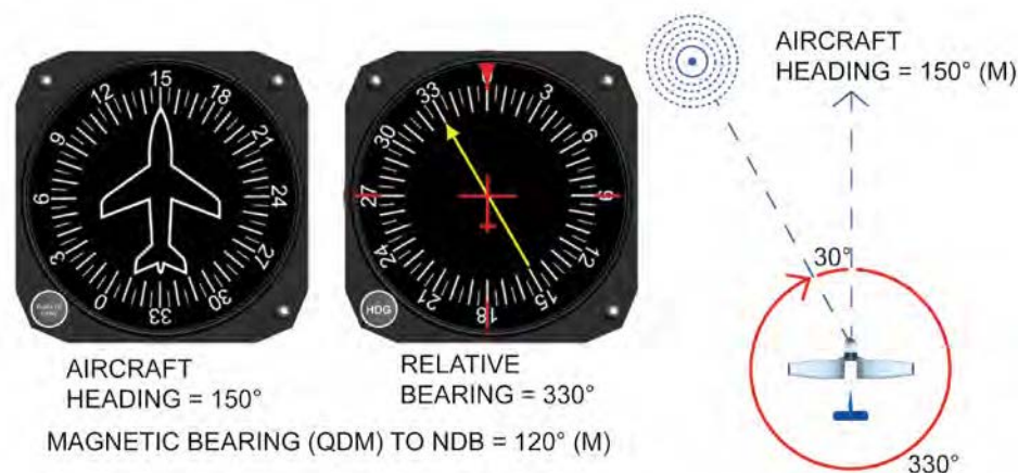
Figure 16.9 With an RBS, the QDM can be read directly from the ADF display.
