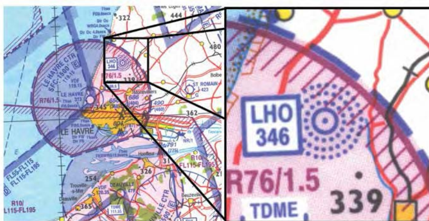
Figure 16.4 The NDB located near Le Havre, in France. Its Morse identification is LHO, and its frequency is 346 KHz.
