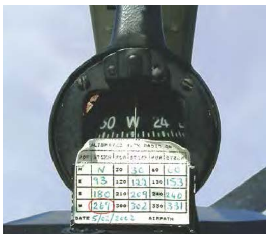
Figure 3.10 Compass Deviation Card, in the form of "headings to steer."
