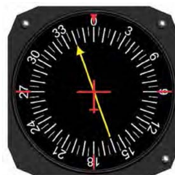
Figure 16.7 An ADF Display, incorporating a Relative Bearing Indicator (RBI).
